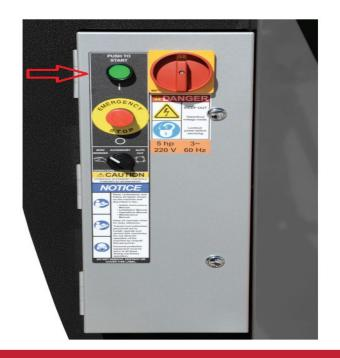
• Emergency Palm Stop - This button de-energizes the machine and contains a manual, safety reset function. The projecting "red" palm stop style button is set within a safety yellow bezel and is pushed to de-energize the machinery. Once de-energized the machine requires the palm stop to be re-set prior to energizing the machine. Simply rotate the emergency palm stop button clockwise. The button will retract and the machine will be available for powered operation.
